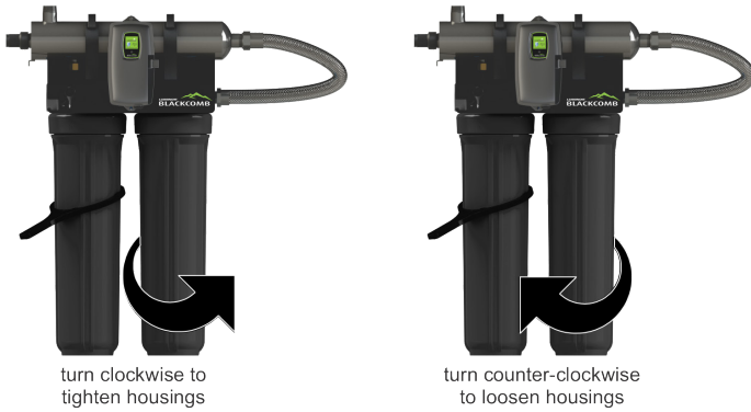
Figure 5. Cartridge Removal
